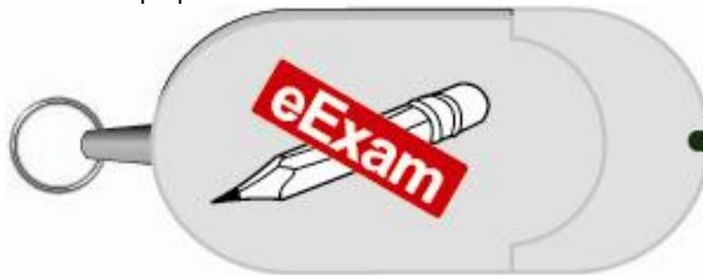
**Each candidate's computer is controlled by this USB stick during the exam, interdicting communications and local disk access.**
